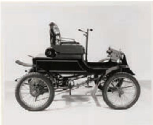
Vehicles had solid axles and carriage leaf springs with no dampers. These vehicles bounced nearly out of control over the rough unpaved roads. As cars got faster the situation got worse.
