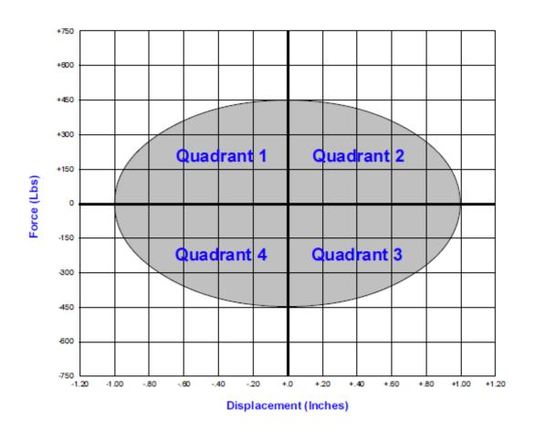
This section of the manual illustrates different valving combinations in the form of graphs. The graph shown is force vs. displacement graph. The force vs. displacement graph is a very accurate and simple way to assess valving characteristics. If you are not familiar with this type of graph, it is explained on the following page along with the graph above, showing the four different quadrants.
