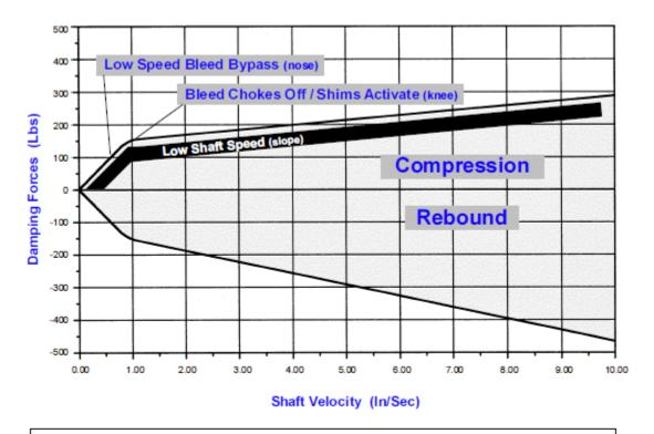
Note: Remember that low speed damping characteristics are controlled by bleed through the low speed adjuster and the bleed hole in the piston, not the valve stacks.
