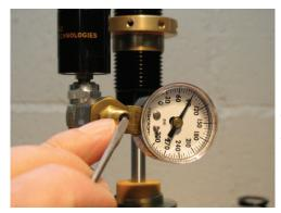
Now turn out the "T" valve and remove the fitting from the shock Schrader valve.
