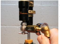
We recommend Nitrogen because it is clean, free of moisture and more temperature stable than compressed air. Using compressed air can introduce contamination and moisture into your shock causing problems with the seals.
